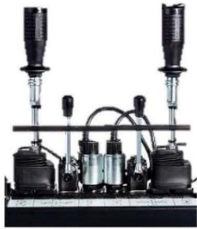
Mechanic control valve, sticks with 2 electric functions
